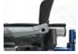
Break lever The folding lever of push to lock brakes makes transfer easier.
