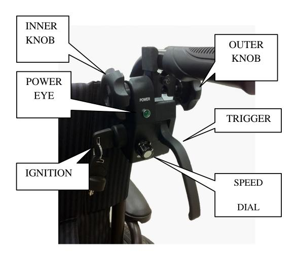
Trigger – Squeeze the trigger to propel the PowerAssist. The more the trigger is squeezed, the faster the PowerAssist will travel. Release the trigger to stop the PowerAssist
