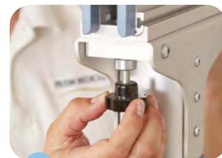
4 Star-Handle securing screws on track section and feet
